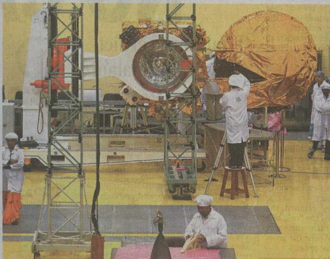
INNOVATIVE FIX: ISRO built the final model of the orbiter from the start instead of building a series of iterative models, as NASA does. Picture shows scientists and engineers working on the Mars Orbiter vehicle in 2013 at ISRO's satellite centre in Bangalore. — PHOTO: AFP
